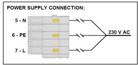
Note: It is important that the Door Operator Module has a good earth connection.
