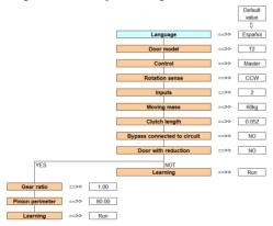
IMPORTAT: If the circuit is turn on, and the Auto-adjustment is pressed, after end the learning process, the circuit will start the Guide Menu. Always a Basic configuration will be necessary to ensure the EN 81-20/50 compliance.
