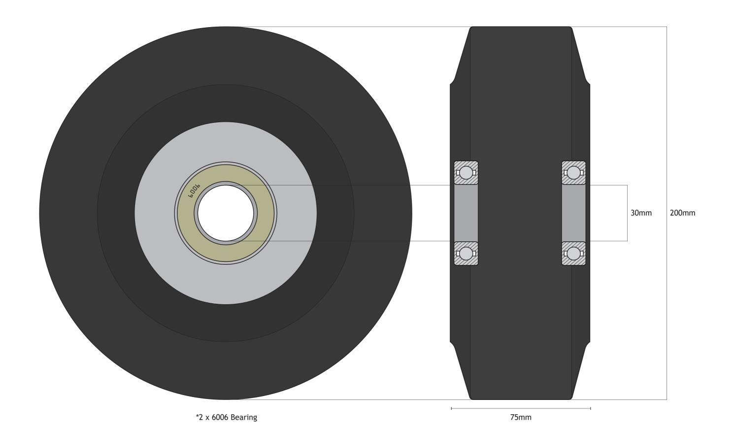
Guide Roller 200mm OD x 75mm Wide with 2 x 30mm Bearings
