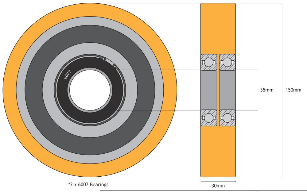
Guide Roller 150mm OD x 30mm Wide with 2 x 35mm Bearings
