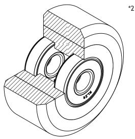
Vulkollan® Guide Roller (75mm OD) VU 92° with Steel Core Date: 4th November 2024 Created by: M. Watkins
