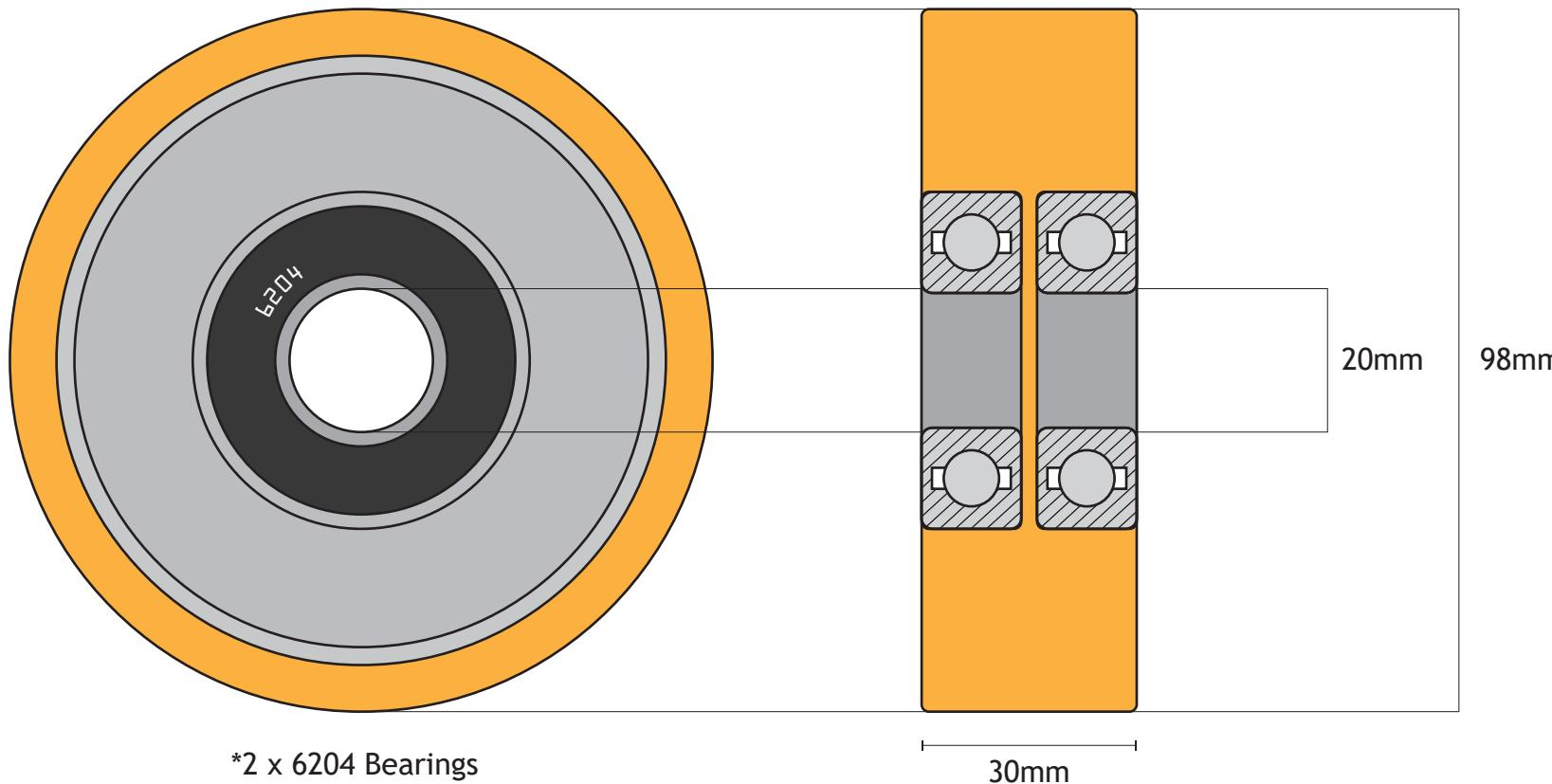
Otis Guide Roller 98mm OD x 30mm W
