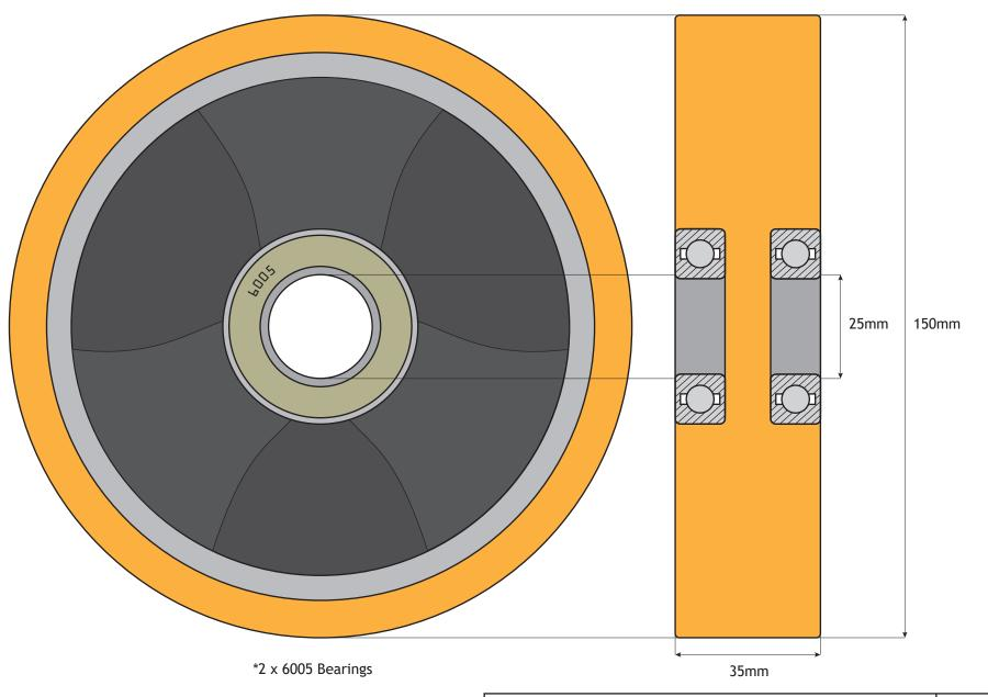
Guide Roller 150mm OD x 35mm W - 2 x 25mm Bearings (6005)
