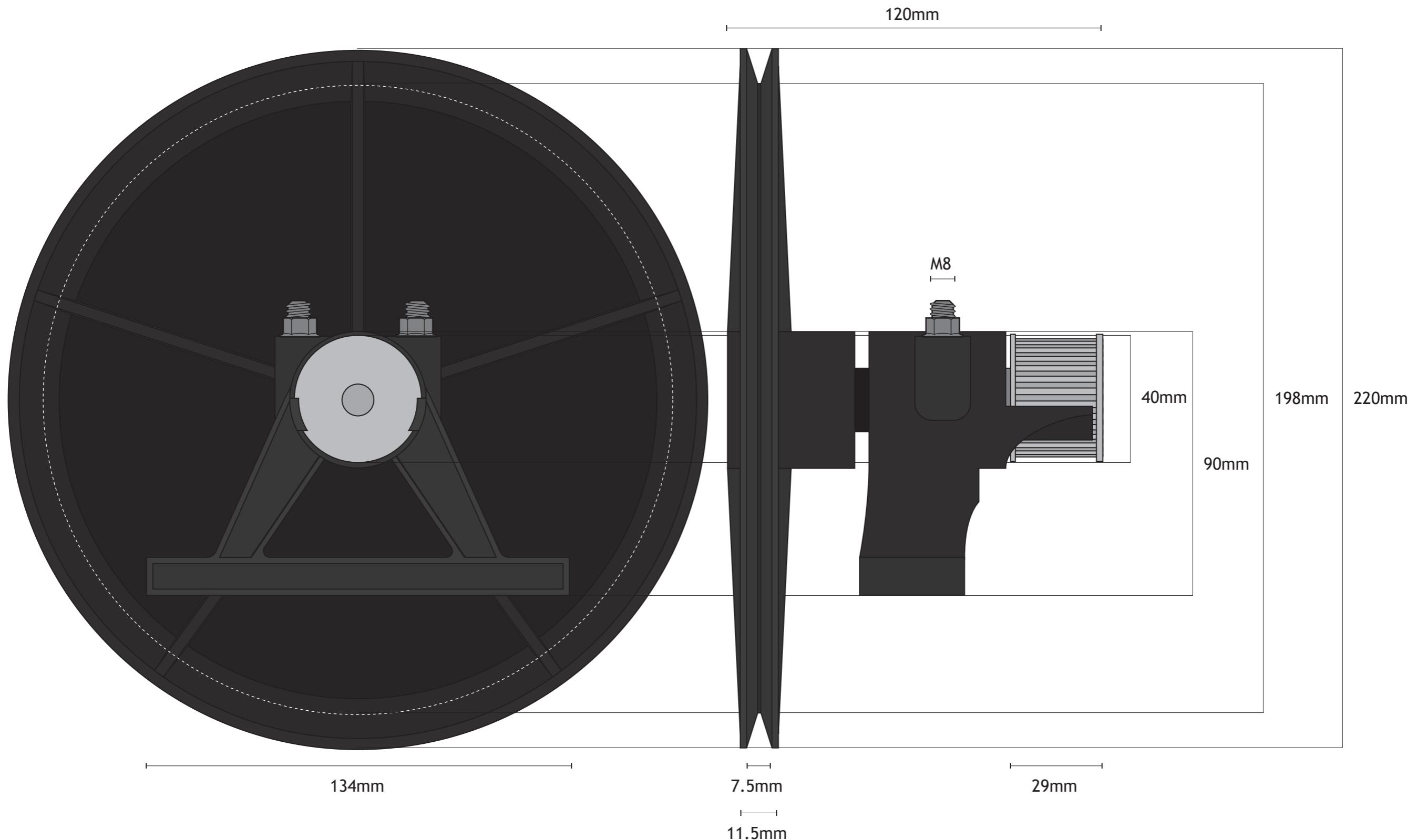
Schindler Reduction Pulley Assembly -
