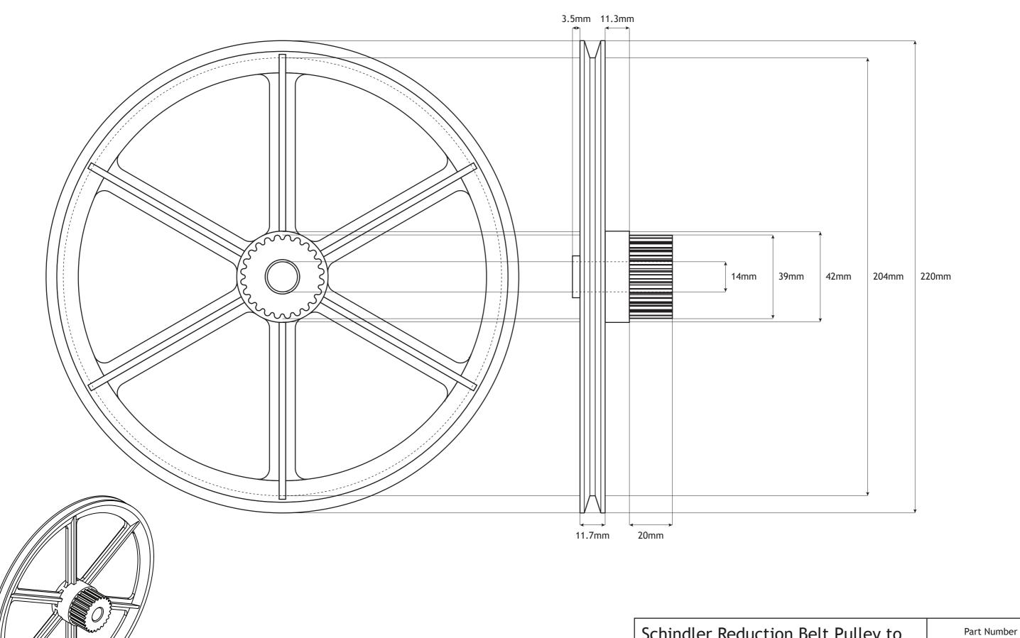
Schindler Reduction Belt Pulley to Suit QKS11 - OEM:830894
