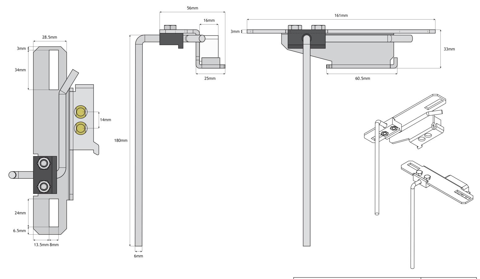
Fermator Lock Release Assembly & Part Number 18704
