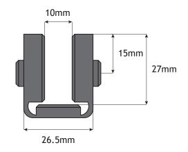
ACLA 100mm Polyethylene Guide Shoe Liner (26.5mm) - 10mm
