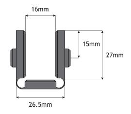
ACLA 100mm Polyethylene Guide Shoe Liner (26.5mm) - 16mm
